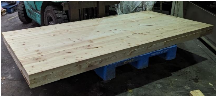
Figure 1: Irish Sitka Spruce CLT panel fabricated on the TERG MODCONS project (2.4 m x 1.2 m x 0.12 m)
